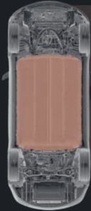
Native electric vehicle, battery-pack architecture example
